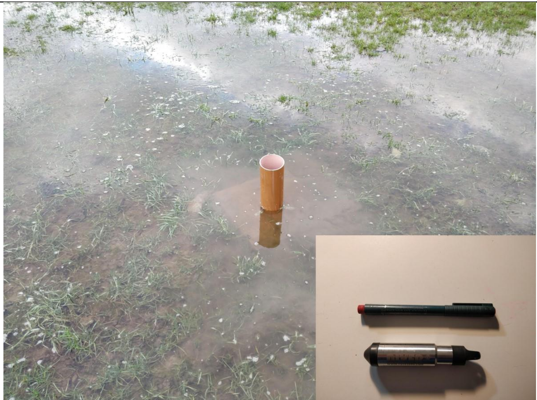
Site Photo 8: Paving slab and ~0.5m pipe used to secure Diver water level logger (bottom right). (Note: This setup was used to monitor water levels in turloughs and in the Ballyglass River)
