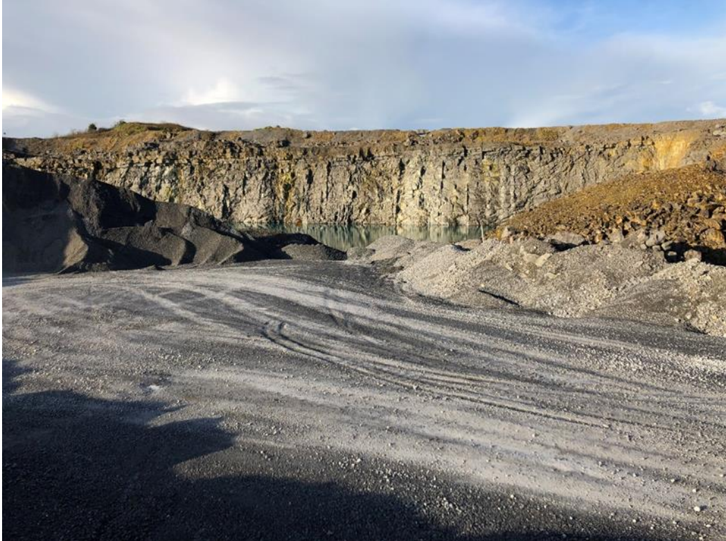
Site Photo 2: Rock face at Cam Quarry. ~15m face with 2-3m of glacial overburden. Rock is strong/competent with little visible fracturing.
